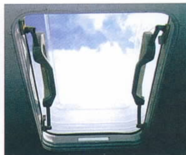
Skylights to lighten up the middle corridor and supply with fresh air
